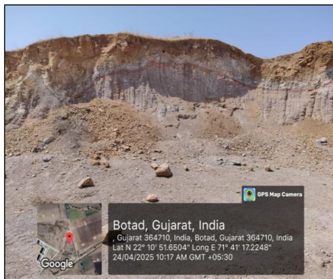
Photograph 6: Exposure of Red bole bed (Act as Marker horizon) near ARTO, Botad
